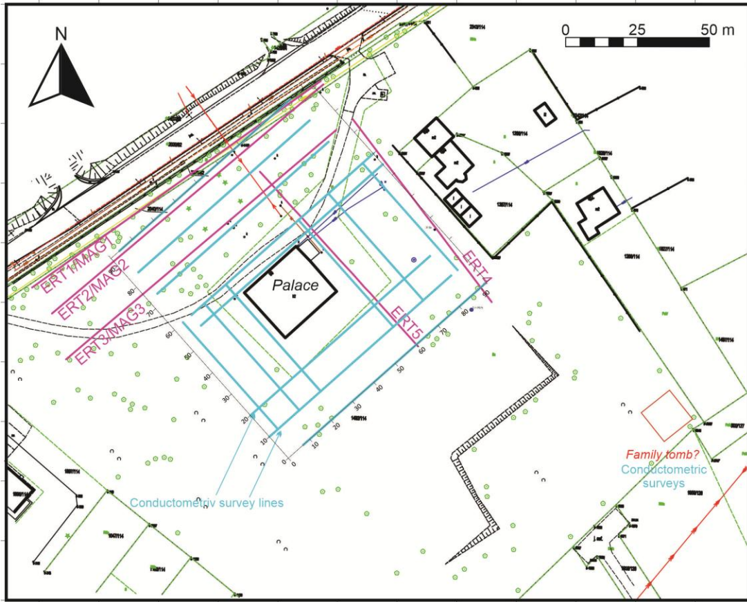
Fig. 2. Geodetic map of the Palace and Park Complex in Rzuchów with survey lines marked
