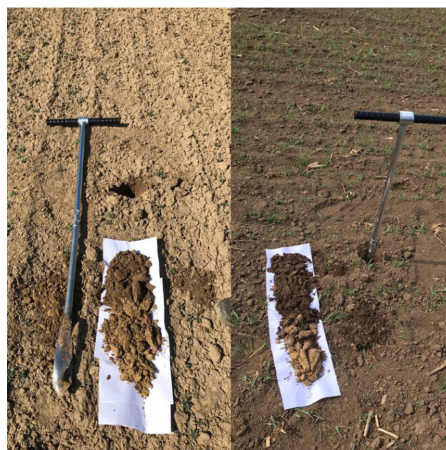
Fig. 2. Edelman verification probe: Haplic Regosol (left); Cutanic Luvisol (right).
