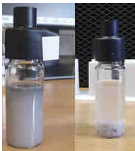
Fig. 9. Comparison of raw emulsion (left) and separated coolant (right) (pH = 10, demulsifier concentration 1 %, stirrer speed 500 rpm, stirring time 10 min)
