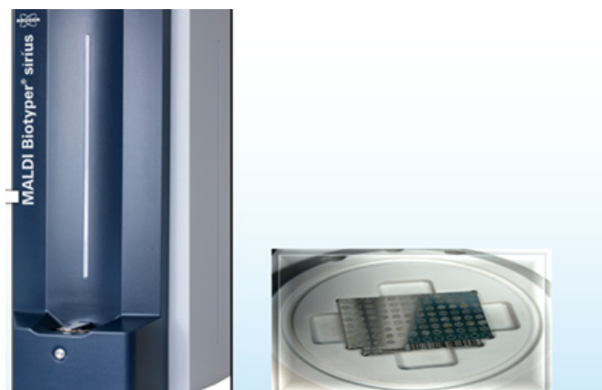
Figure 2. The colony are placed on a MALDI target plate in order to be identified. The device irradiates the target plate with a laser. Compass software automatically generates MALDI-TOF Spectrum. To identify the sample, the acquired MALDI mass spectral fingerprint is compared with the stored database.
