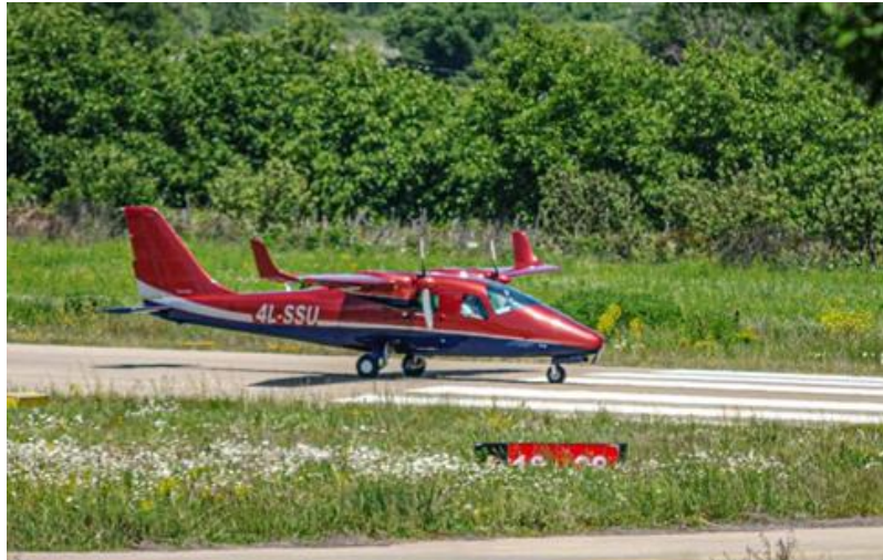
Fig. 10. Tecnam P2006T (MTOW 1230 kg, Max cruise speed 269 km/h)
