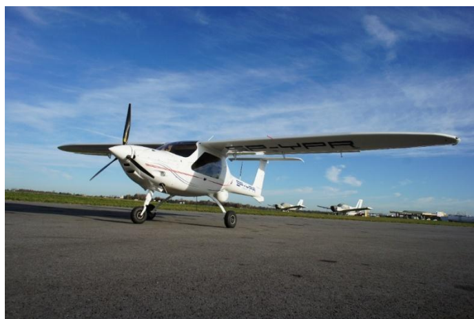
Fig. 5. Optionally Piloted Vehicle (MTOW 495kg, Max. Airspeed 270 km/h,
