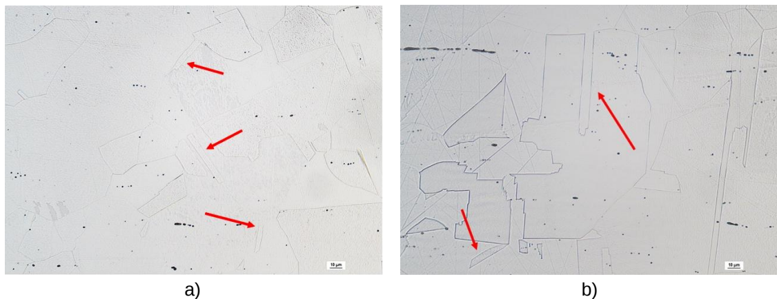
Fig. 3. Microstructure of austenitic stainless steel; a) AISI 304, b) AISI 316L, etc.
