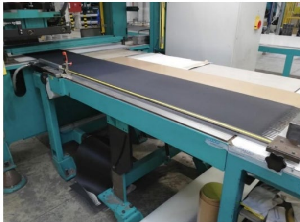
Fig. 4. New placement of material when cutting out joints after the introduced changes (Binčík, 2022)
