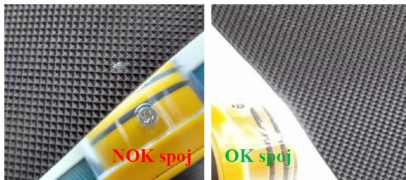
Fig. 11. The part of the SOP defining a link fault (Binčík, 2022)
