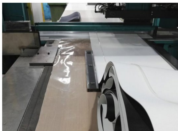
Fig. 3. The original placement of the material when cutting out the joints before the changes were introduced (Binčík, 2022)
