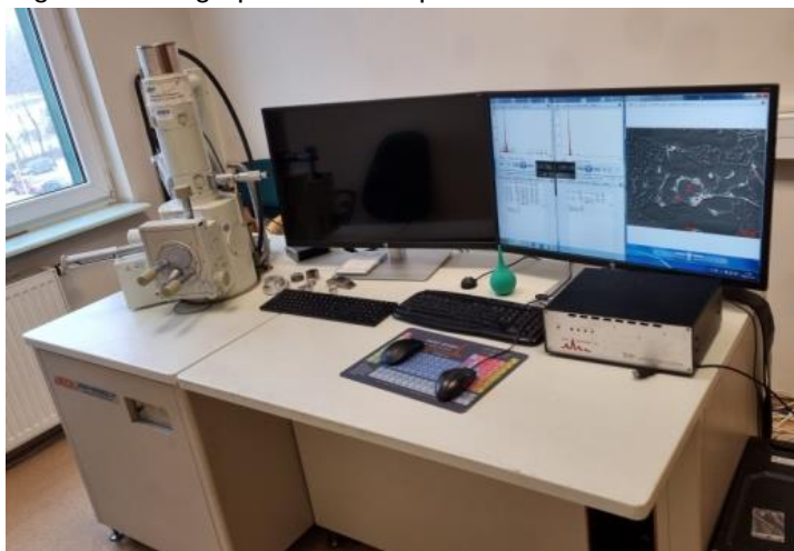
Fig. 3. Electron scanning microscope Jeol 5600LV with built in X-Ray Microanalyzer EDS 2000
