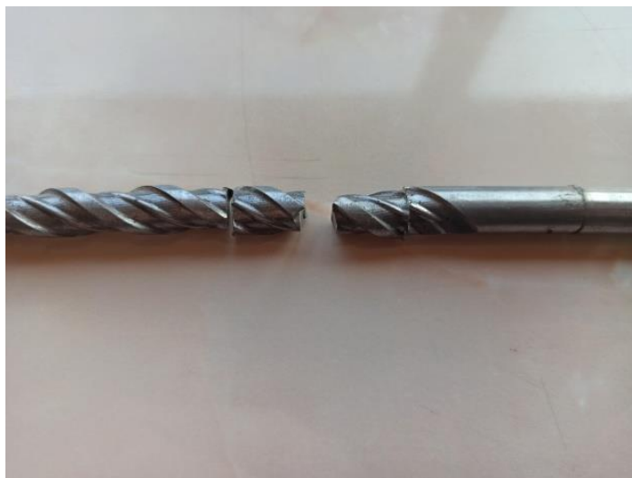
Fig. 1. Macro image of the drill bit damage location
