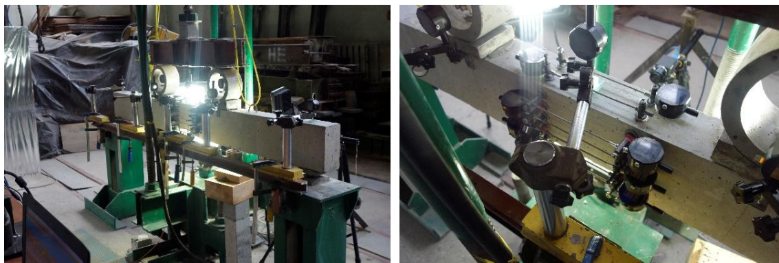
Fig. 5. General view of the experimental setup and the location of the devices on the test reinforced concrete beams
