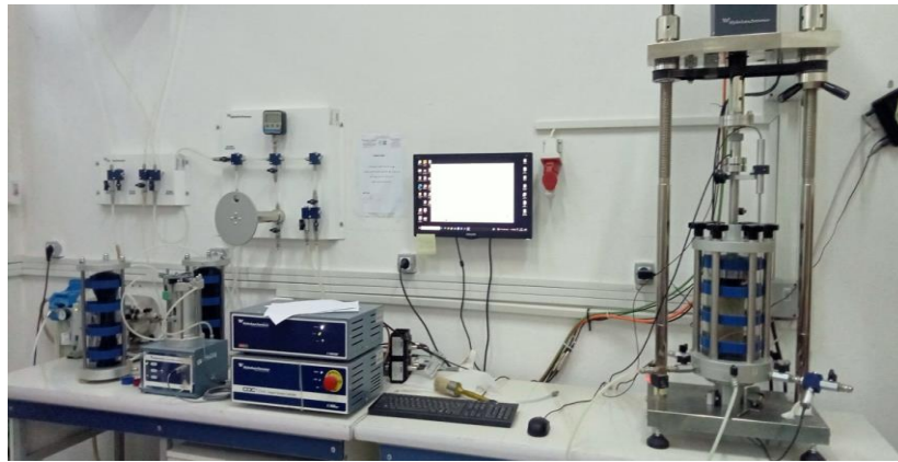
Figure 3: The triaxial device used for monotonic and cyclic testing (DYNATIAX EmS)
