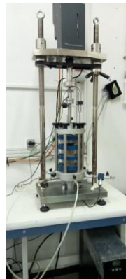
Figure 4: Cyclic triaxial pressure cell (DYNATIAX EmS)
