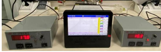
Figure 5: Oxygen diffusion testing apparatus
