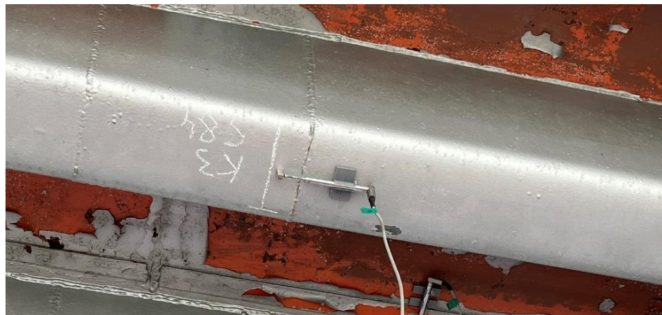
Figure 10: LVDT placement at Section 84 - horizontal
