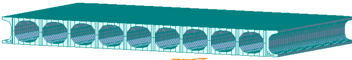
Figure 4: Structure displayed with cross-section thicknesses and shapes
