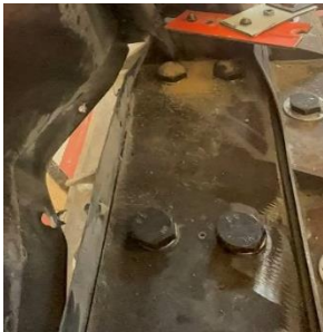
(d) Pull-out of the sheathing from the fasteners head - Experimental results
