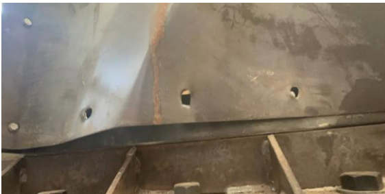
(b) Pull-out of the sheathing from the fasteners head-Experimental results.
