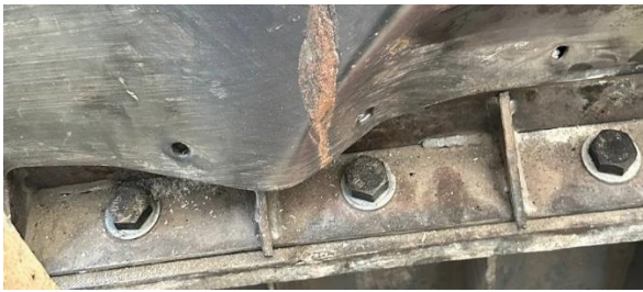
(a) Pull-out of the sheathing from the fasteners head-Experimental results
