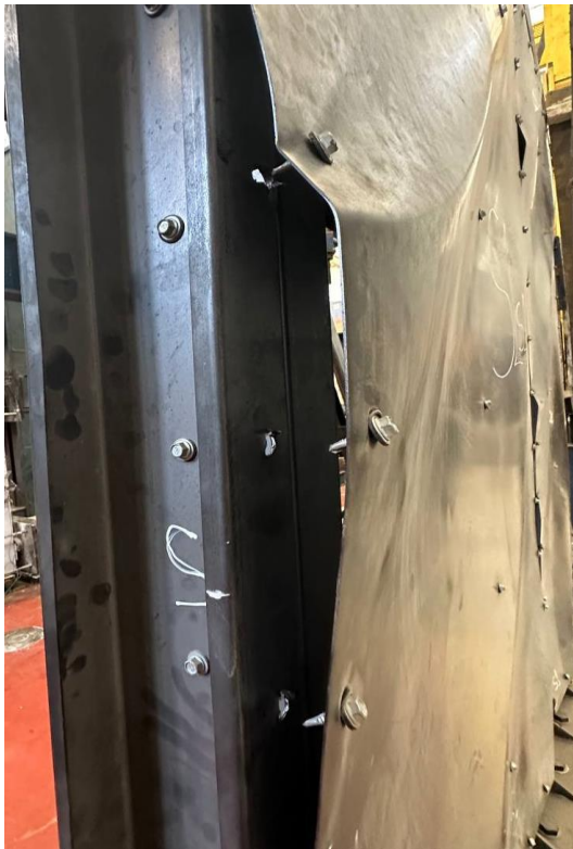
(a) Screw full-out failure mode- Experimental test
