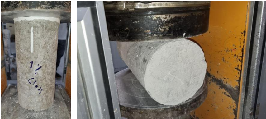
Figure 3: Compressive and Splitting tests by the universal testing machine
