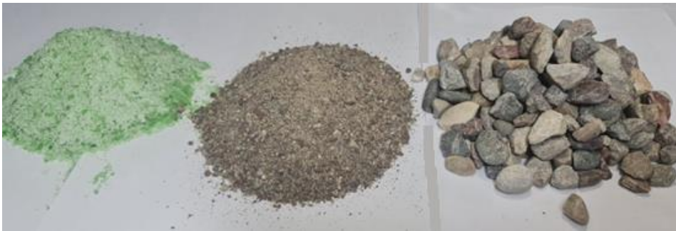
Figure 2: Sample of recycled glass, fine aggregate, and coarse aggregate
