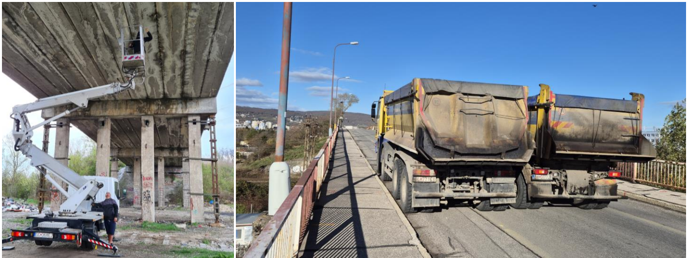
Figure 11: a) Detailed inspection of critical sections, b) the most unfavourable position of the load during the load test
