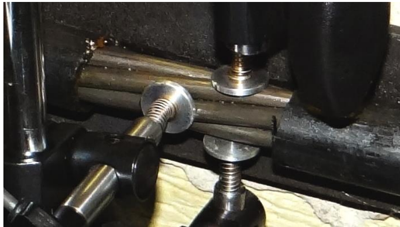
Figure 6: Three inductive sensors for measuring strand displacement and flattening (Svoboda & Klusáček, 2018)
