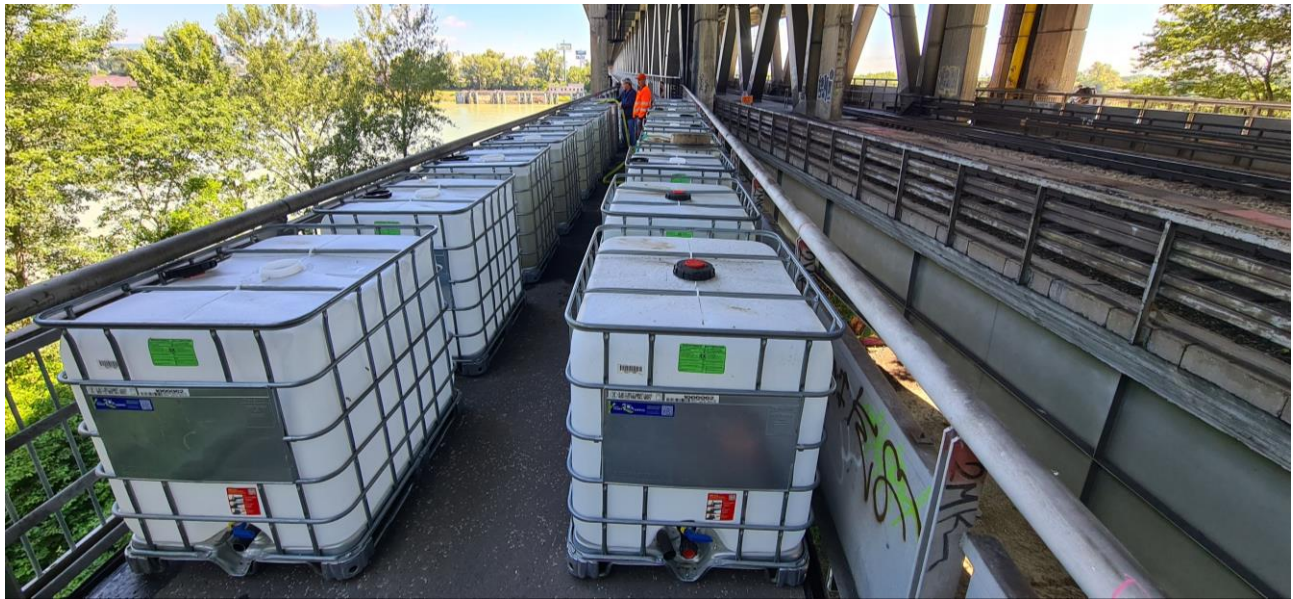
Figure 5: Plastic tanks used as testing load
