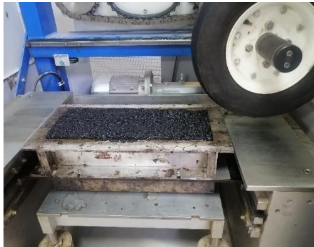
Figure 4: Roller compactor with compacted plate
