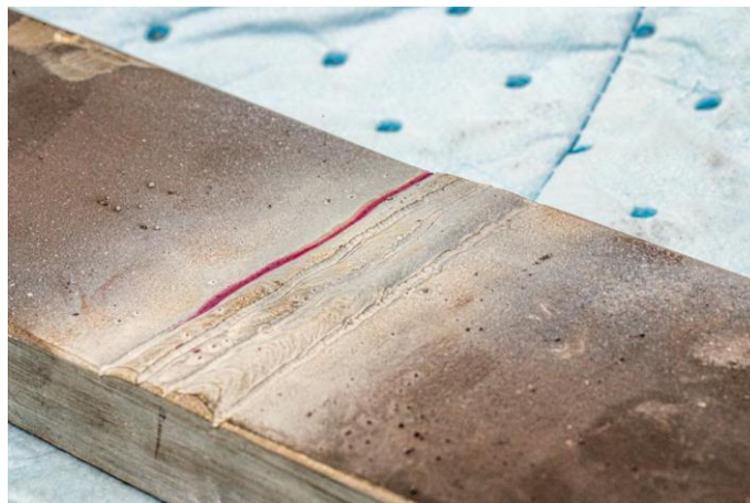
Figure 5: Localization of the fatigue crack using NDT penetrant testing (PT) after completion of loading
