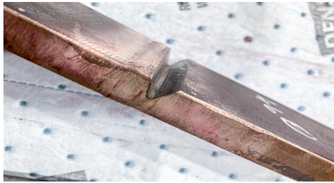
Figure 6: Repair of a specimen affected by a fatigue crack
