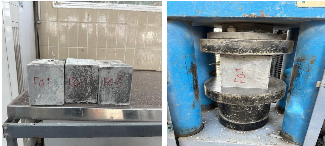
Figure 5: Compressive Strength Test
