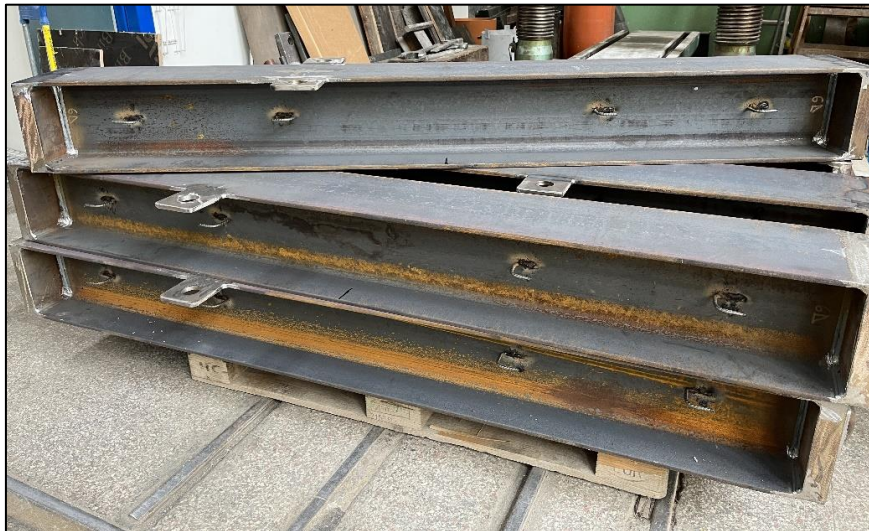
Fig. 5: Prepared steel columns with welded shear connectors prior to concrete infill casting.
