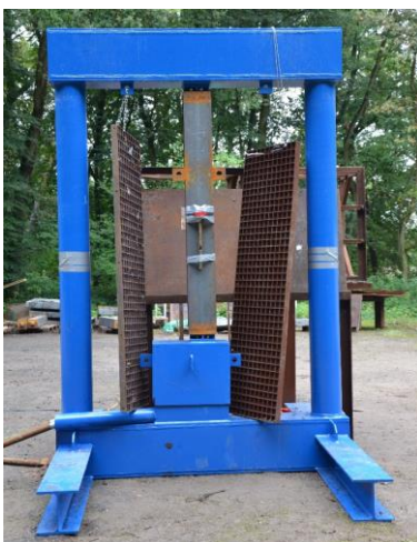
Fig. 10: Steel testing frame with the mounted column specimen before the blast test.
