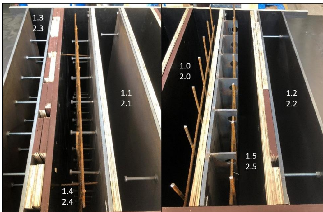
Fig. 3: Formwork arrangement for the casting of slab specimens.
