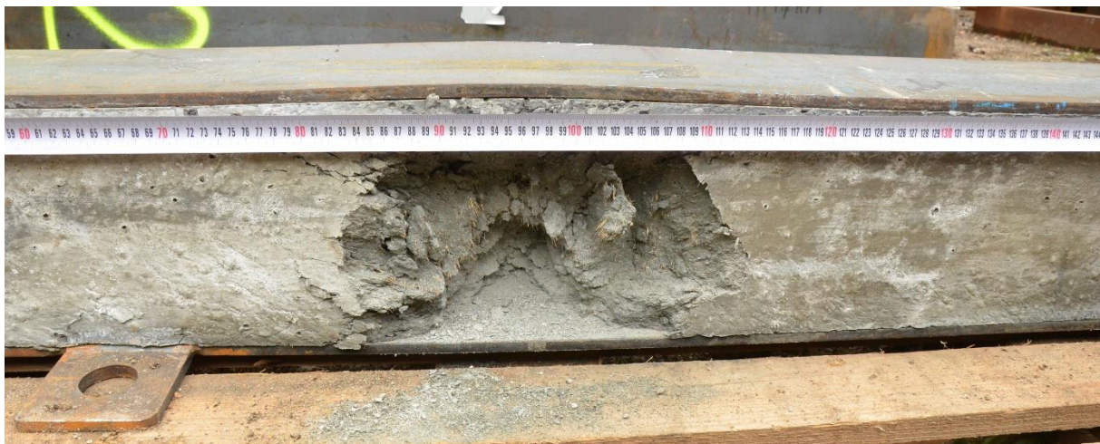
Fig. 22: Side view of composite specimen with UHPFRC infill (type 3).
