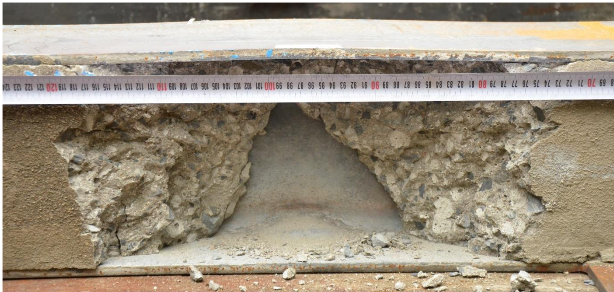
Fig. 21: Side view of composite specimen with NSC infill (type 2).
