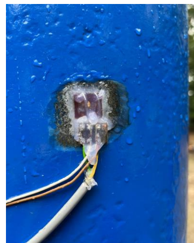
Fig.11: Placement of strain gauges along the side of the steel testing frame.
