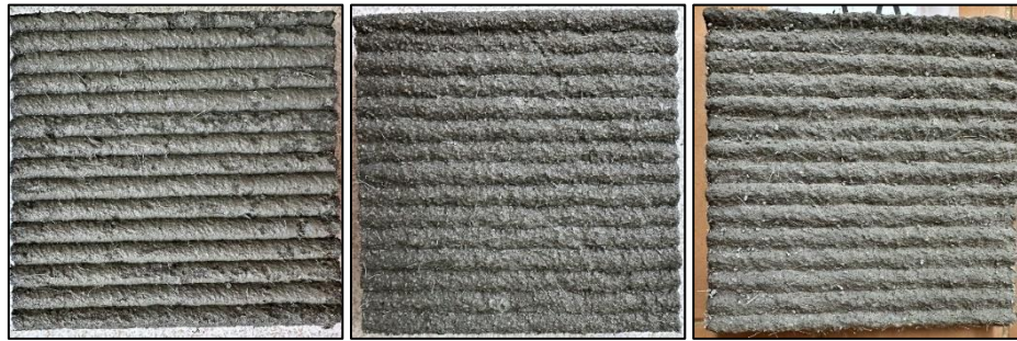
Fig. 9: Specimens after 100 F-T cycles – method A (From left to right: PE sheet 28d, PE sheet 3d, No PE sheet).
