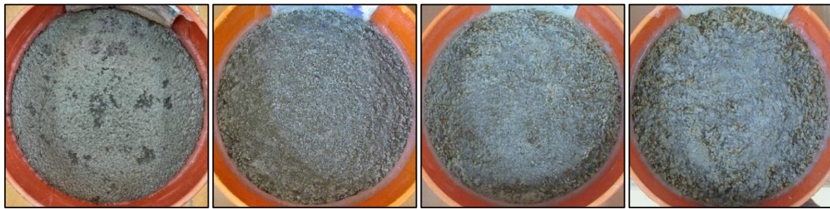
Fig. 7: Specimens after 75 F-T cycles – method C (From left to right: REF, REF-ACC, SFIB, SFIB-ACC).
