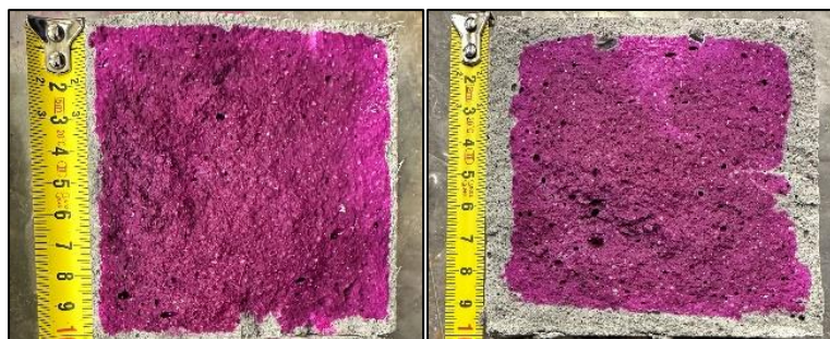
Fig. 14: Test specimens (From left to right: 7 days and 28 days in CO 2 chamber).
