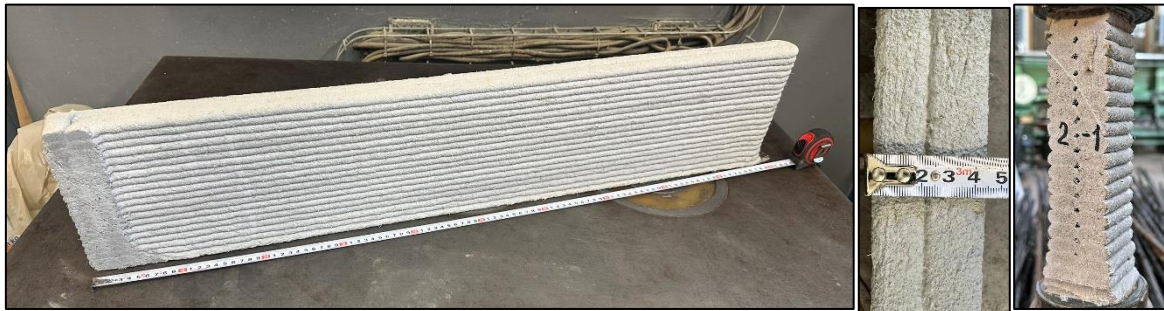
Fig. 4: The 3D printed double wall with imperfect connection.
