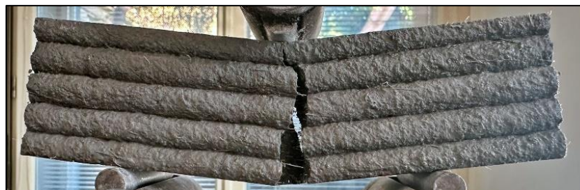
Fig. 12: Flexural test - failure mode.
