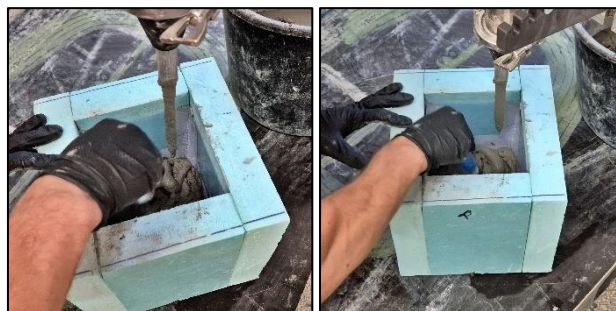
Fig. 6: Method of filling molds for some types of tests performed.
