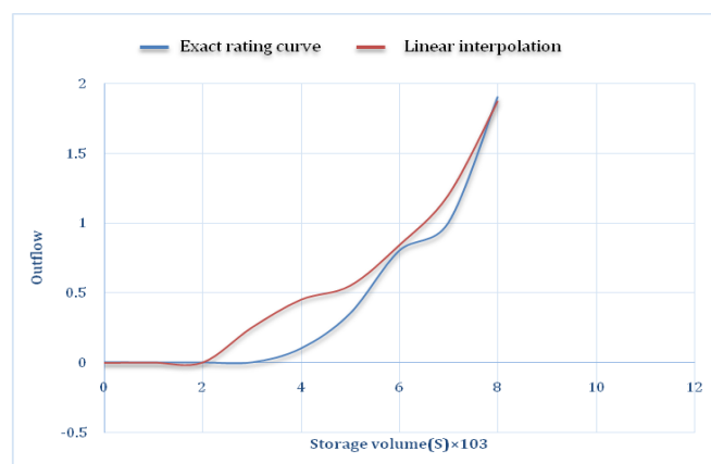
Fig. 1: The relation between storage and outflow.
