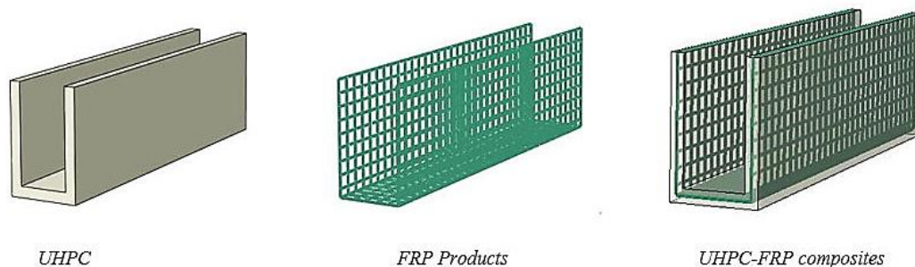
Fig. 10: The formation of UHPC-FRP composites.
