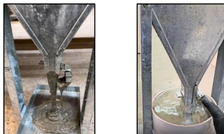
Fig. 3: V-funnel test (conventional and underwater).
