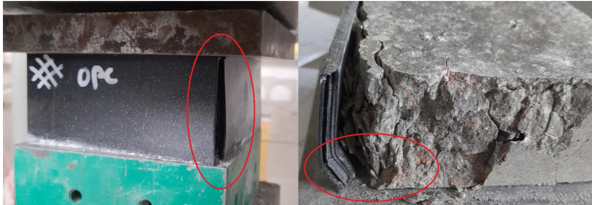
Fig. 4: The nature of the failure of the OPC specimen in the mould with a reinforcing grid.
