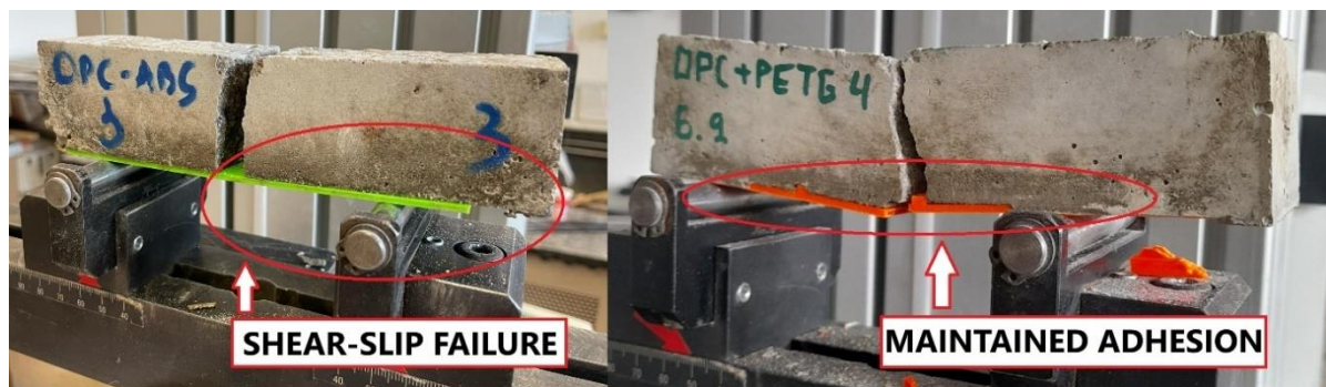
Fig. 7: Adhesion distortion while maintaining the integrity of the plain ABS polymer element in the OPC variant (left) and adhesion preservation of the PETG element and OPC part in the case of failure of the specimen by flexural testing.
