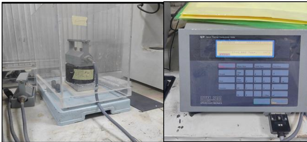
Fig. 3: The QTM-500 Quick Thermal Conductivity Meter used for measuring the thermal conductivity of materials.
