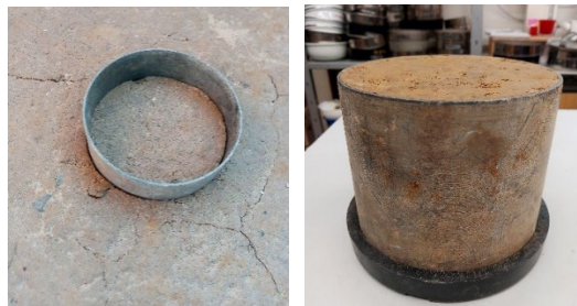
Fig. 4: Sampling to evaluate the basic characteristics of the subgrade.
