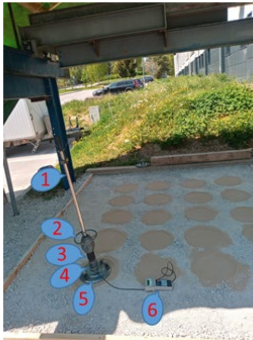
Fig. 8: Dynamic load test set and locations of the experimental stand.
