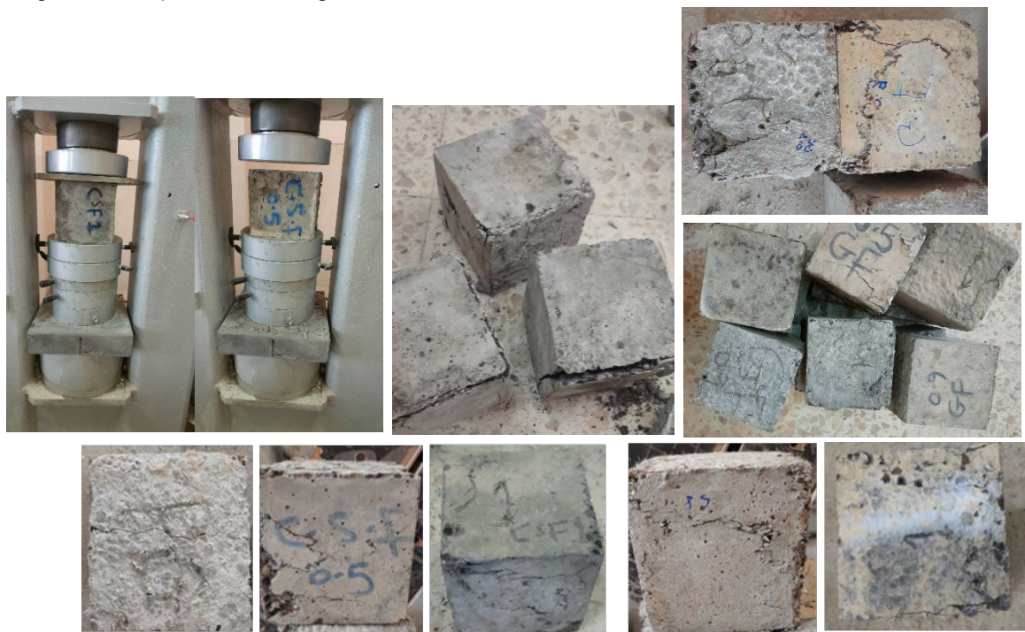
Fig. 5: cubes specimens test and failure shapes
