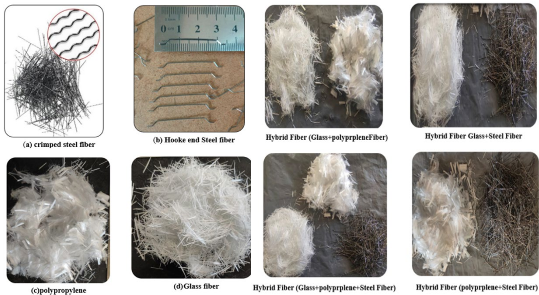
Fig. 1: Type of fiber: a – single fibre , b – hybrid fibre
