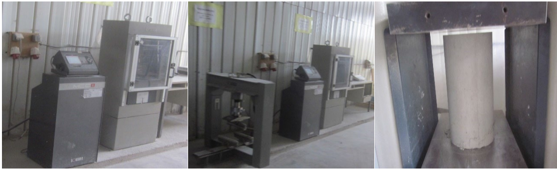
Photo 2: The testing equipment used to determine the compressive strength of cylindrical specimens.
