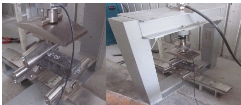
Photo 1: The testing equipment used to assess the flexural strength through a three-point bending test.
