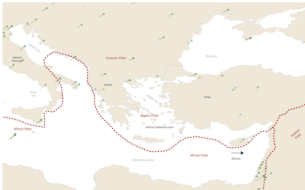
Fig. 8: Horizontal shifts of permanent observation space geodesy stations (ITRF2020) in the locality of Balkan peninsula (Authors), Tectonic plates boundaries source [38]
