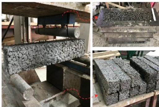
Fig. (5). Flexure strength for prism
