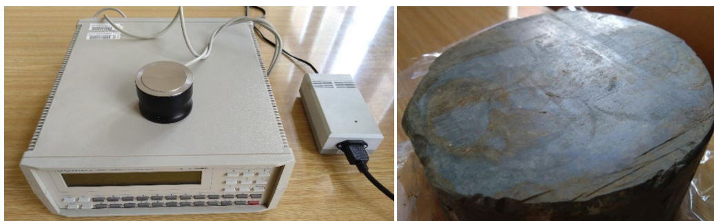
Fig. 2: Isomet 2104 device with surface probe and specimen of Neogene clay.
