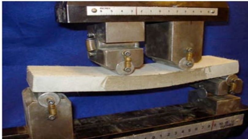
Fig. 5(b). ECC-PVA Concrete specimen showing large deflection under modulus of rupture test.
