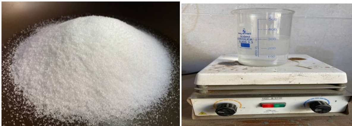
Fig. 8 (a). PVA Powder. (b). PVA Powder after Dissolved, derived from experimental Mix Proportion of ECC-PVA Concrete.
