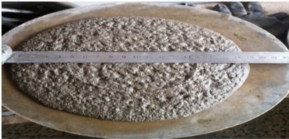
Fig. 9. Flow Table Test.
