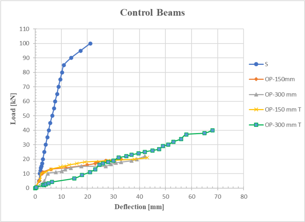
Fig. 9: Load-mid span deflection relationships for control beams.
