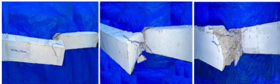
Fig.32: Cracks pattern at failure for OP-300T beam.
