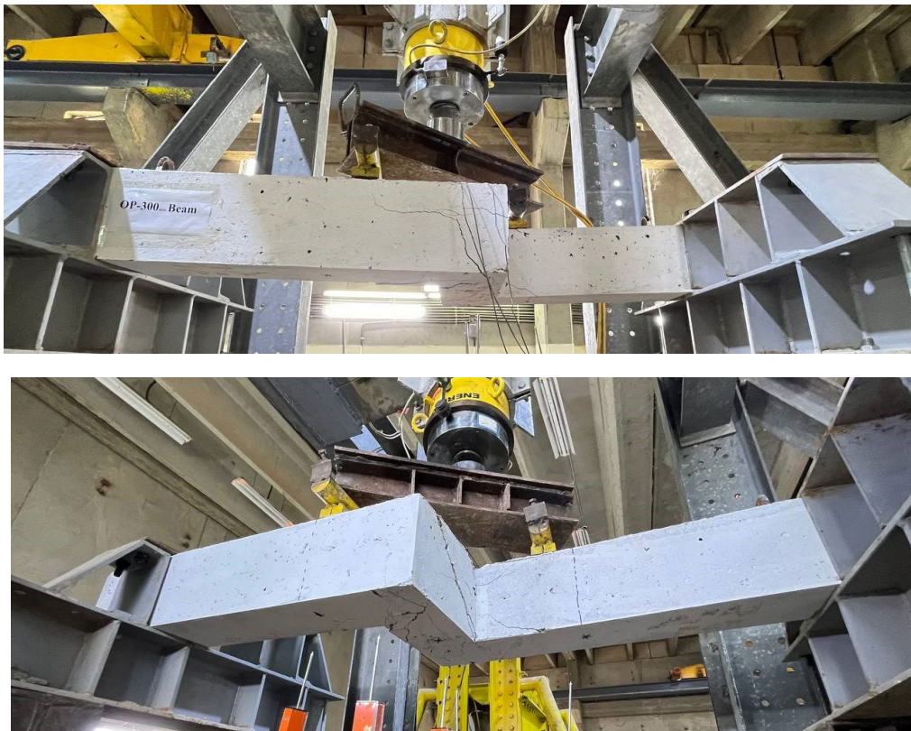
Fig. 5 The applied load details.
