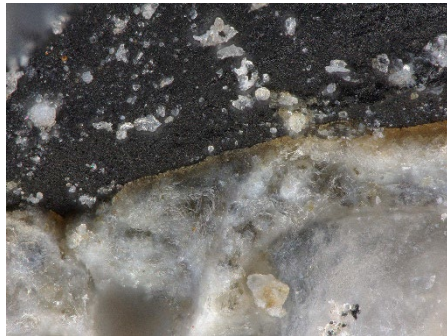
Fig. 15: The interface between rubber granules and cementitious matrix [20],
