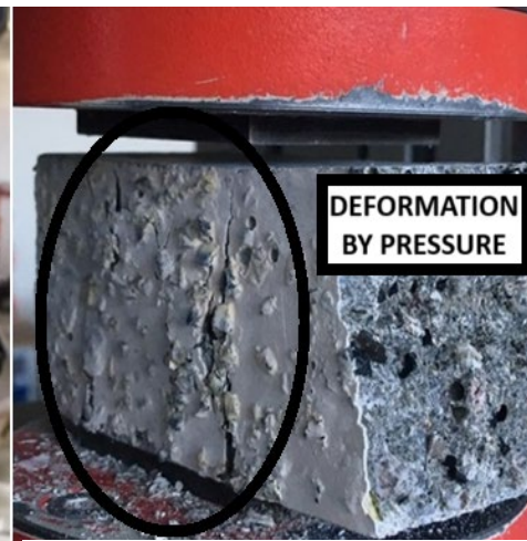
Fig. 5: Specimen failure after compressive strength test with load area of 40x40 mm [16].
