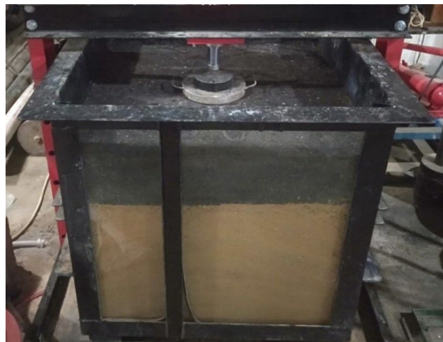
Fig. 6: A performance of the plate loading test on subgrade stabilized
