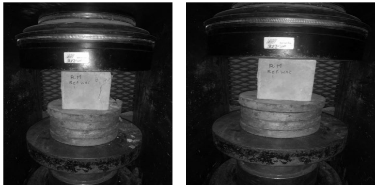
Fig. 3: Reference mix concrete during test for compressive strength.
