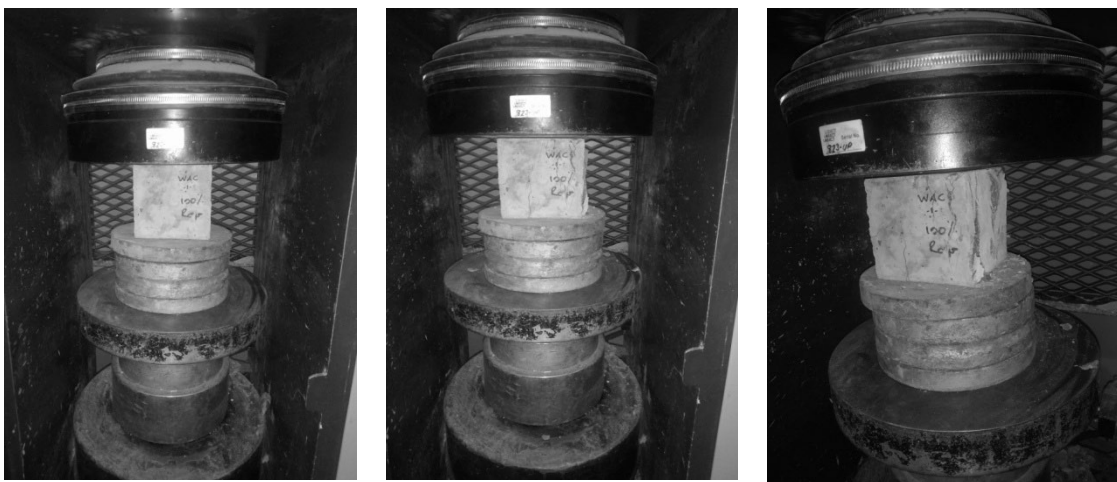
Fig. 4: Concrete contain waste concrete aggregate during the test.
