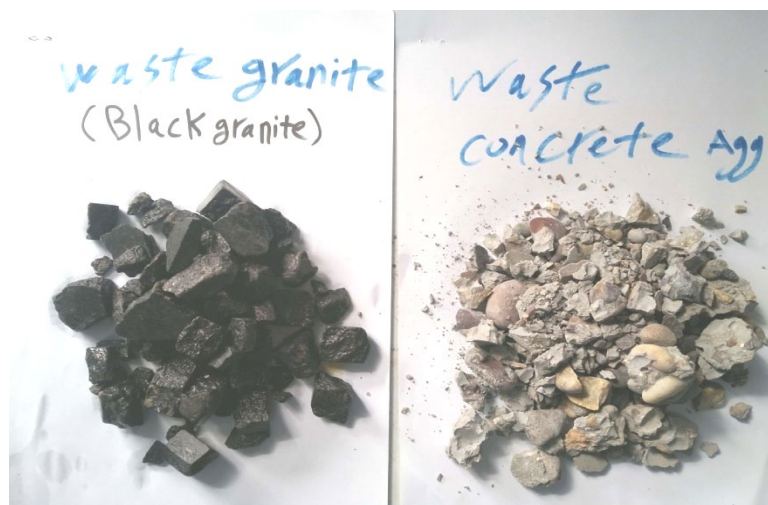
Fig. 2: Illustrative picture for waste concrete aggregate and waste black granite used in the study.
