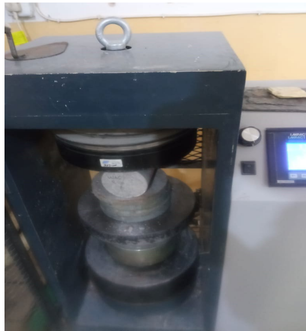
Fig. 6: Waste granite aggregate concrete under the tensile test.
