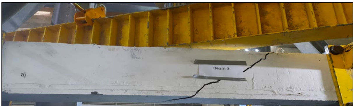
Fig. 13 Cracks Pattern in Beam BW
