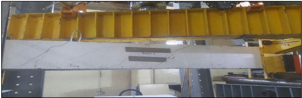
Fig. 13 Cracks Pattern in Beam BW
