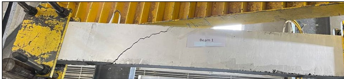
Fig. 12: Cracks Pattern in Beam BN
