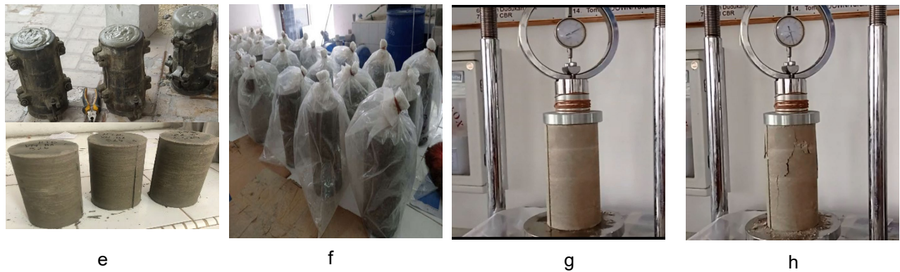
Figure 1. (a) Mortar Construction, (b) Foam Production, (c) berat busa , (d) Flow Test, (e) Cylinder Samples, (f) Maintenance, (g) Compressive Strength Test, (h) After Compressive Strength Test
