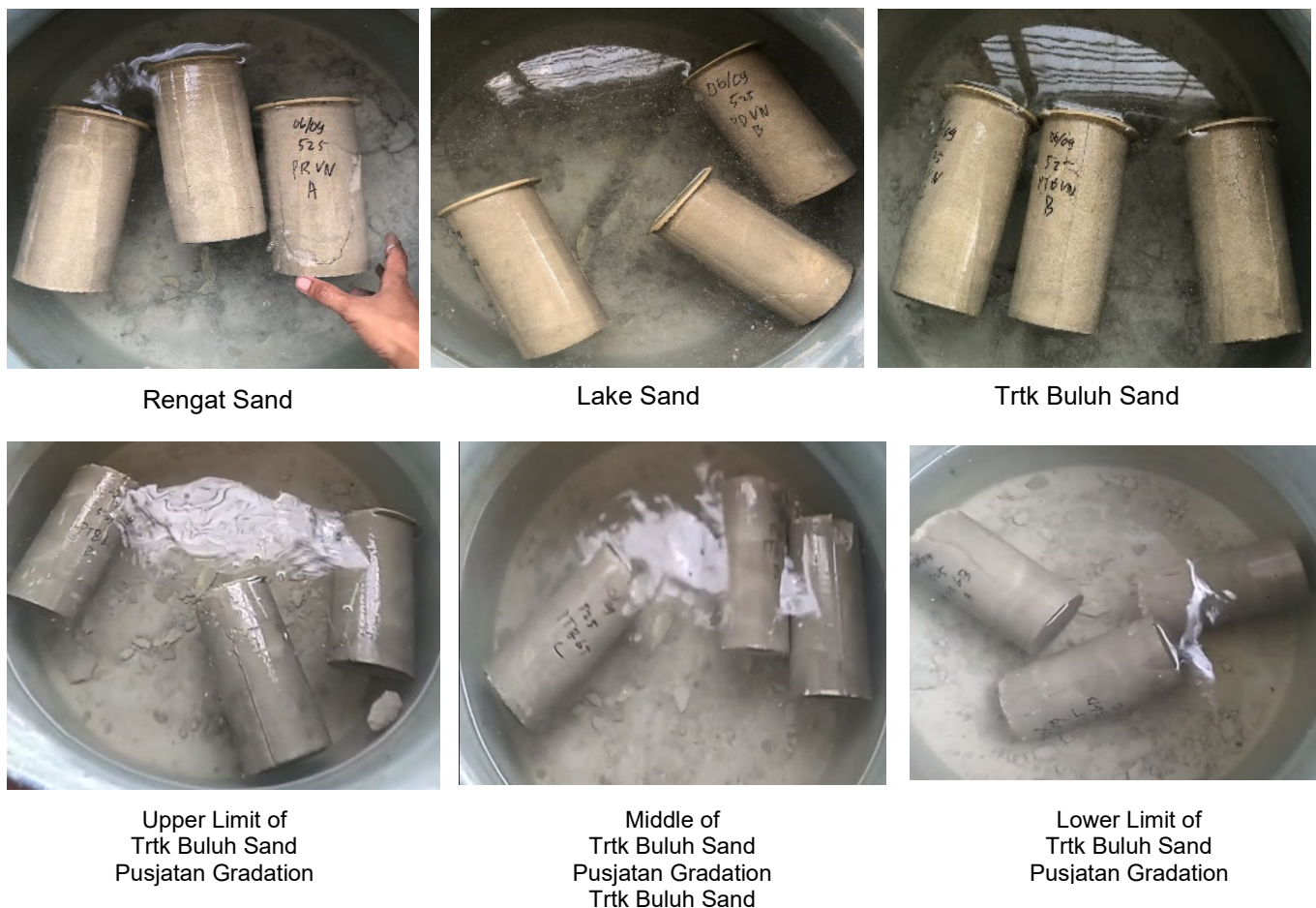
Figure 6. FMLT samples, six gradations in water
