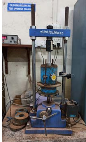
Fig. 3: Laboratory set up for the mobilized bearing capacity test.
