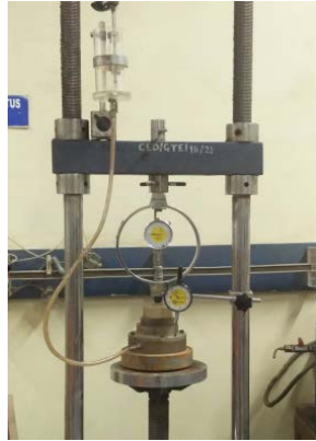
Fig. 1: Laboratory set up for the swelling pressure test.
