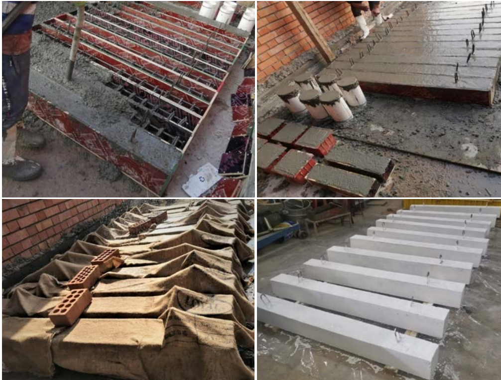
Fig. 2: Casting, curing method, and beam specimens.
