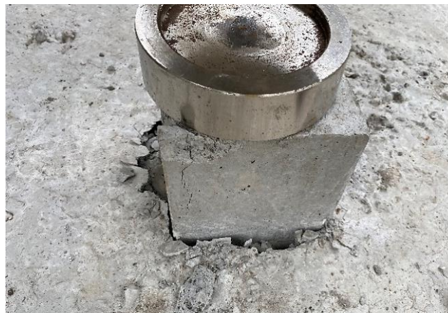
Fig. 6: Punching shear at the centre of the tested voided flat slab.
