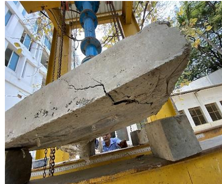
Fig. 19: Yield line crack pattern of voided flat slab (Final crack).
