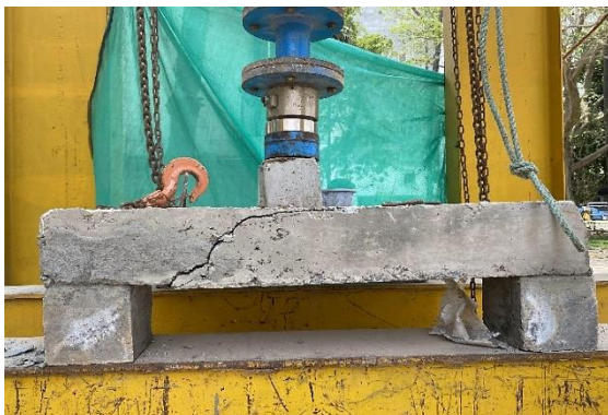
Fig. 20: Yield line crack pattern of voided flat slab (36VS8).
