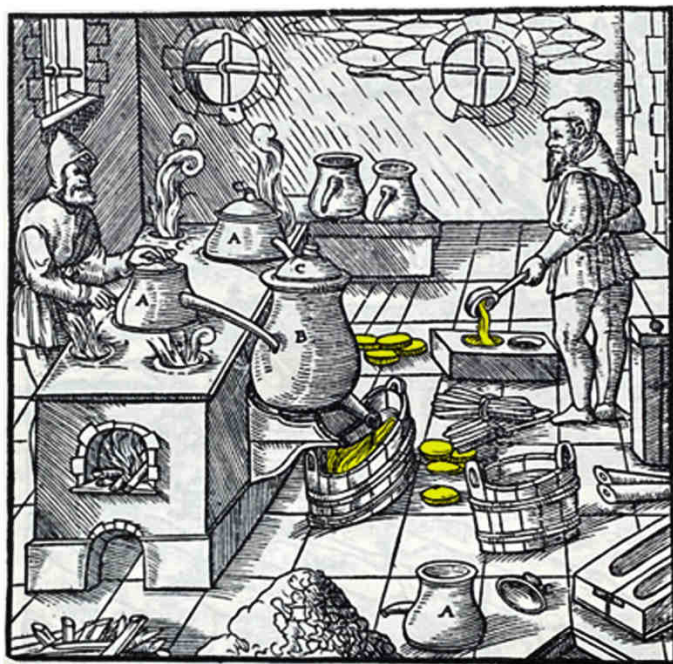
Fig. 6. Purification of sulphur
