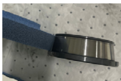
Figure 2. The grinding of the bearing raceway
