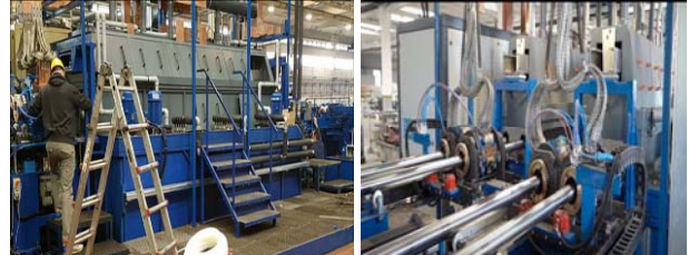
Figure 12. Continuous chromium plating installations with a single chromium plating cell [25,26]
