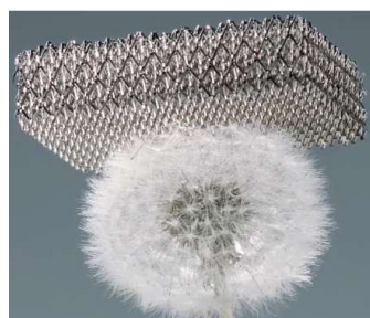
Figure 9 Ultra-lightweight sandwich panels based on nano-crystalline metals standing on the dandelion [92]
