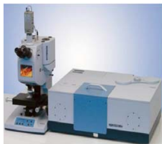
Figure 5. IR spectrometer with fourier transform (FTIR) coupled with a high resolution IR microscope
